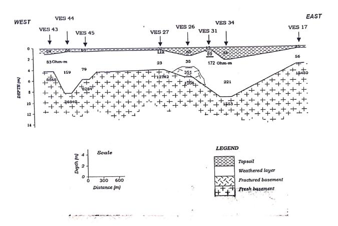
Figure 1: Cross Section of Interpreted Resistivity Data
